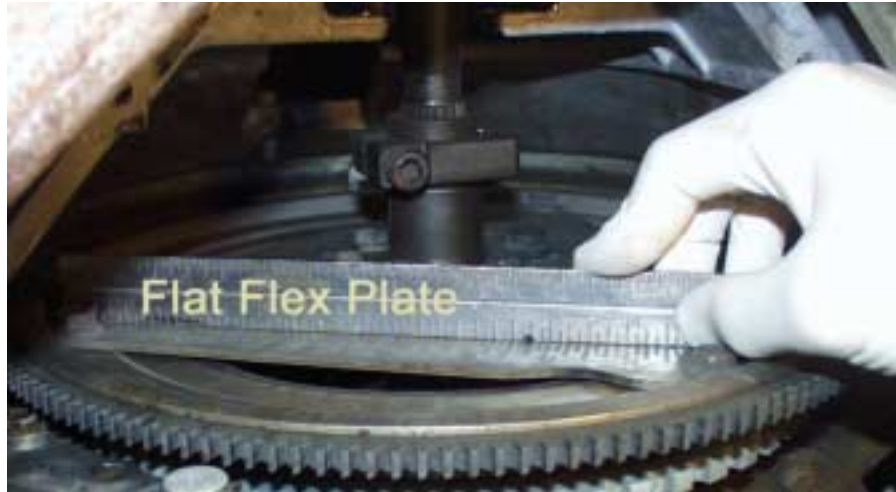
Figure 8. Flex Plate with no Tension.
