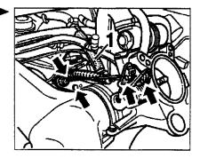
10. Remove the center and right vent hose on the throttle body.
