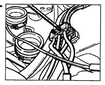
17. Fasten the wiring harness using the two rubberized clamps.
