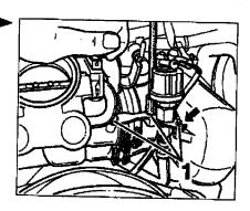
25. Engage accelerator cables -arrows-. Lightly oil the rubber of the accelerator cables. Tighten the accelerator cable holder. Connect the hose -1-. Ensure that the accelerator cables are seated correctly and tightly.
