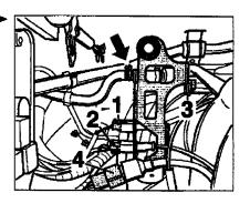
Disengage the accelerator cables -arrows- and unscrew the screw of the counter holder. Press the accelerator cables out of the holder. Pull off the hose -1-.
