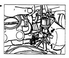
12. Pull all vacuum connections and connectors on the intake distributor. Remove the vent hose -1-. Mark the vacuum connections.
