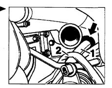
31. Pull wiring harness up and out. Doing this requires a second person. One person must press the wiring harness from below through the opening in the engine compartment while the other person pulls the wiring harness out.
