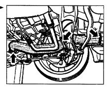
26. Remove the transmission vent hose and suction hose to the tur-bocharger. To do so, release the upper screw-type hose clamp-arrow- and the lower clamp -arrow-.
