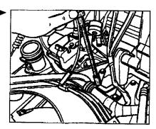
97 52 55 Replacing the wiring harness for the turbocharged engine Printed in Germany, 2002 993-Turbo
