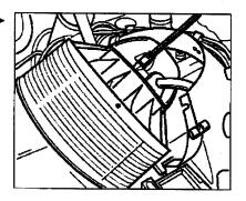
Install the cooling fan and tighten the restraining strap with a hexagon socket head bolt.
