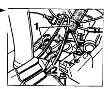
97 52 55 Replacing the wiring harness for the turbocharged engine Printed in Germany, 2002
