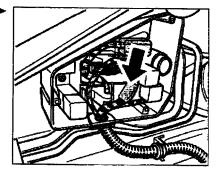
**97 52 55** Replacing the wiring harness for the turbocharged engine Printed in Germany, 2002 993-Turbo
