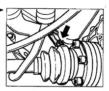
28. Release the connections from the starter -1 + 2- and cut off the 2 tie-wraps -arrow-.
