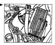
Unscrew the generator housing screws. Release the cable from the generator. Press the rubber grommet out of the air cowl and pull out the lines.
