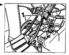
23. Connect the center and right vent hose on the throttle body.
