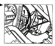
13. Remove the complete intake distributor (right, left, and center)
