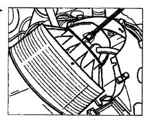
20. Release the ignition wire retainer and unclip the fastening clip.
