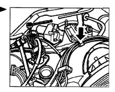
15. Release the ground cable from the intake pipe.
