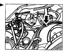
Tightening torque 10 Nm (7.5 ftb.).
