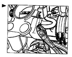
24. Place the oil pressure sensor holder and tighten the screws - 1-. Fasten the ground strap -arrow-.
