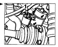
29. Pull out reversing switch connector. To do this, pull out the rubber grommet and the two pins.
