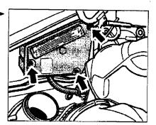
5. Check the part number of the wiring harness. The part number is affixed to the wiring harness -arrow- in the relay carrier in the engine compartment. If one of the following part numbers has been printed on the wiring harness or if the part numbers can no longer be read, the wiring harness for the engine must be replaced.
