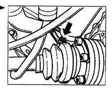
Install the transmission vent hose and suction hose to the turbocharger. To do so, fasten the upper screw-type hose clamp -arrow- and the lower clamp -arrow-.
