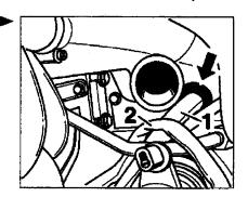
Lightly lubricate the rubber grommet -arrow- of the wiring harness and press it in. Ensure correct seating.
