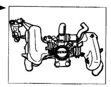
22. Connect all vacuum connections and connectors on the intake distributor.
