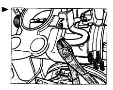
11. Unscrew the screws -1- of the oil pressure sensor, disconnect the connector and disconnect the ground strap -arrow-. Lay the oil pressure sensor aside.
