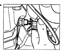
4. Fasten the ground cable **-arrow-** on the starter. Tighten the hexagon socket nut.
