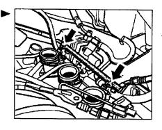
12. Guide the generator connection cable through the air cowl and press in the rubber grommet. Place the cable on the generator, lubricate slightly, and fasten. Press rubber grommet in the air cowl. Position generator cover and tighten.
