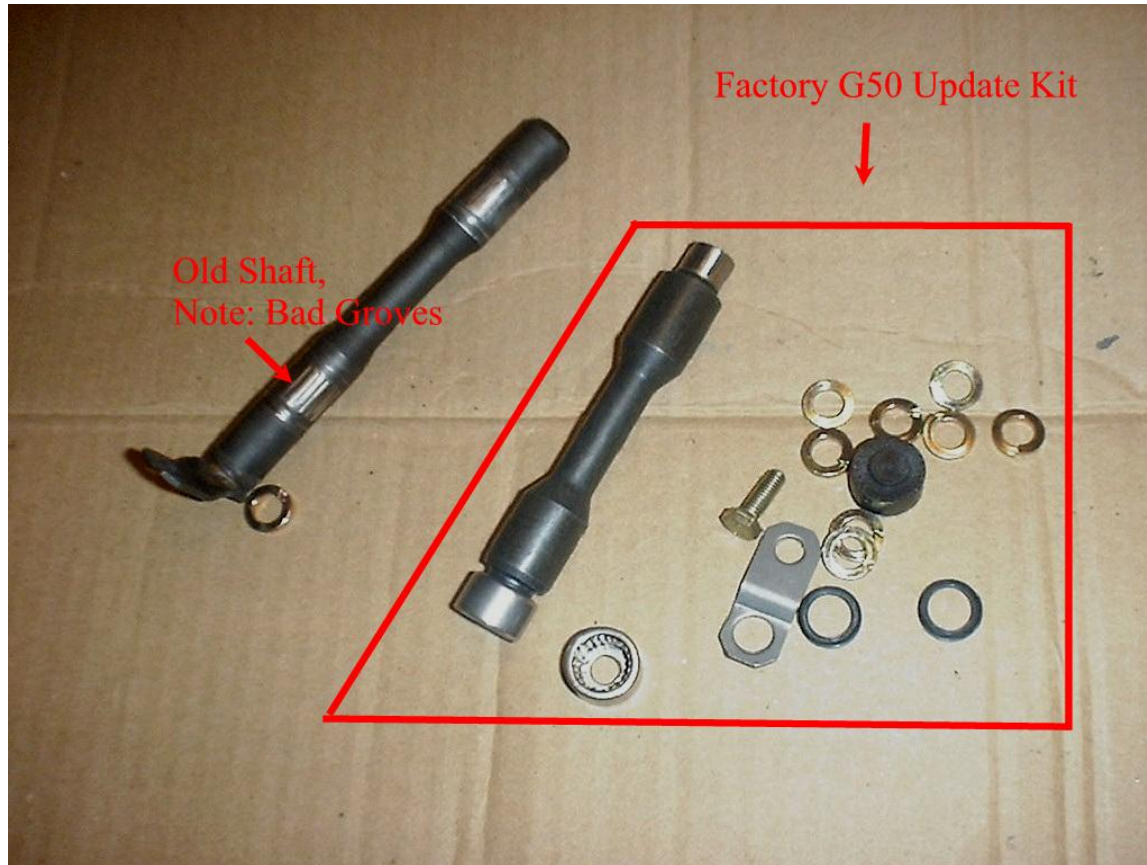
Figure 1 – Factory G50 update and old Shift Fork Shaft
