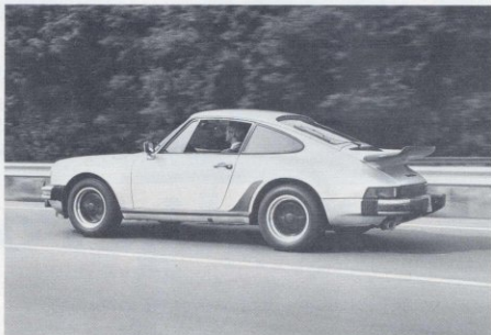
Turbo's fenders are even wider than the normal Carrera's, as are tires and track.
