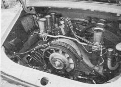
In the 911S an air cleaner and an air-conditioning compressor almost hide the engine. In the Carrera RSR you can see the works.
