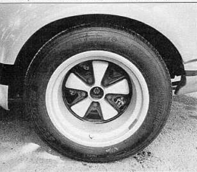
Carrera RSR details: large fuel tank, Space Saver spare and cross brace leave no room in front compartment; cross-drilled brake discs from 917 can be seen through 11-in.-wide rear wheels.
