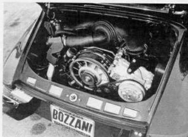
In the 911S an air cleaner and an air-conditioning compressor almost hide the engine. In the Carrera RSR you can see the works.
