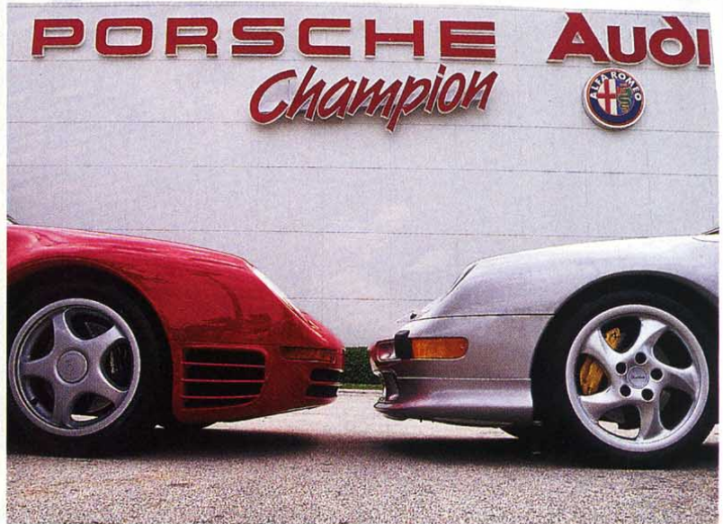
The extensive air ducting in the 959's nose feeds a water radiator in the center and twin oil coolers in either corner.
