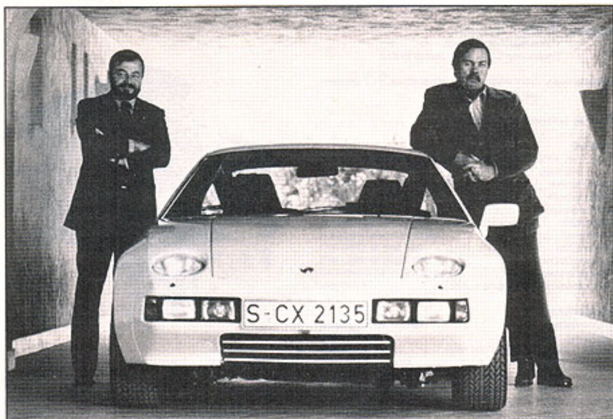
Yates: Tony Lapine, on the left (with David E. Davis, Jr.), is the man who created the 928 shape. Unlike so many high-performance automobiles, the 928 needs only a small chin spoiler at the front (although a faster, turbocharged version will need more aerodynamic aids). Thankfully, the high-style plastic nose will meet U.S. bumper standards without awful alternatives.
