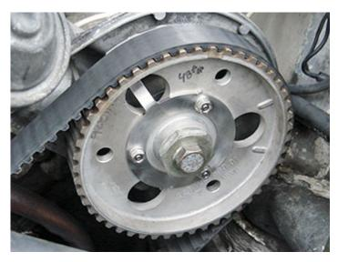
Install 8mm nuts and hand tighten.
