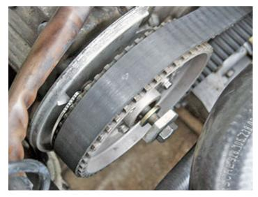
Repeat adjustment procedure on right cam.
