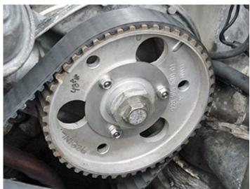
Rotate crankshaft two revolutions until  $0 \mid T$  is again indicated. Check adjustment. Repeat as necessary.
