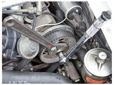
Counter hold the shoulder washer with 32mm wrench while loosening or tightening cam bolt.
