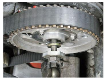
Loosen and remove 17mm cam bolt and shoulder washer.
