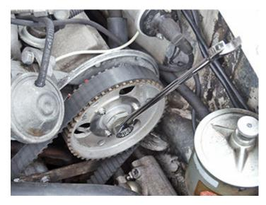
Tighten 8mm nuts. Remove and reinstall cam bolt **without** spacer and using torque wrench, tighten to specification.
