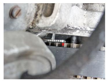
Turn crankshaft clockwise slowly until  $0 \mid T$  is indicated on balancer and pointers are aligned with housing marks.
