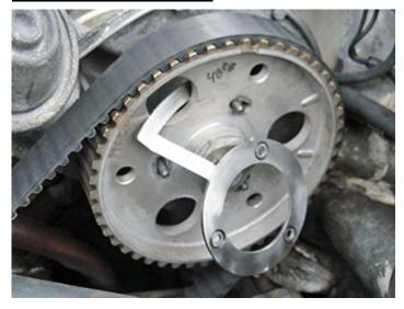
Turn crankshaft clockwise past TDC until notches on cam gear are straight up.
