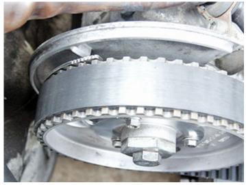
The slightly larger notch on the pointer arm is zero. Each notch is 2 degrees. Clockwise advances, counter-clockwise retards.
