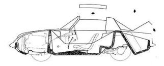
The common goal: a one-piece, self-sustaining, fail-safe, corrosion resistant and dröhnfreier vehicle body, which are both light, as is also stable. In addition, he should be able to be built with minimal tooling costs and provide an appropriate basis for an experimental car, that too.
