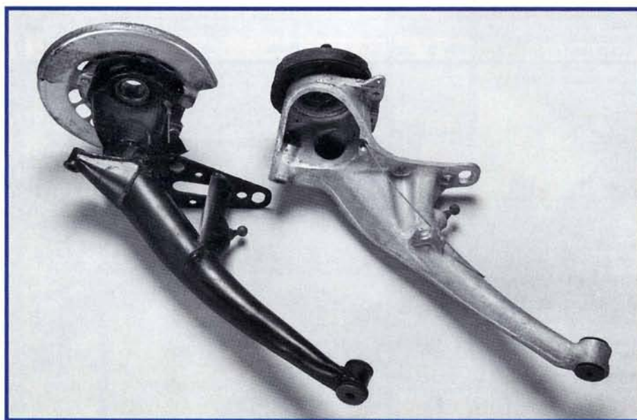
Figure 4—1972-73 steel arm (left), 1974-77 alloy arm (right). Except for a larger diameter shock mount, this is a near bolt-on replacement.
