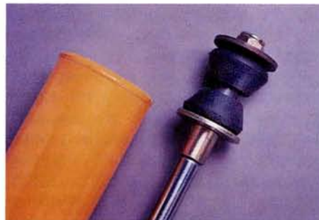
Figure 7—For additional space, discard dust shield and replace with steel washer as a base for upper shock mount hardware.
