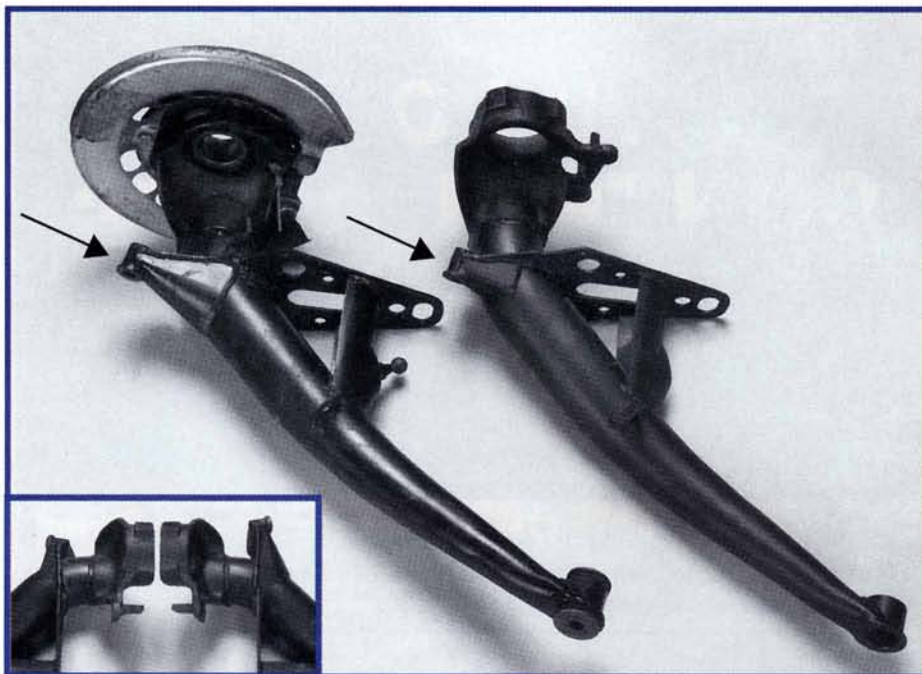
Figure 3—1972-73 (left) and 1969-71 (right) steel arms. Note difference in lower shock mount. Arms are otherwise identical.
